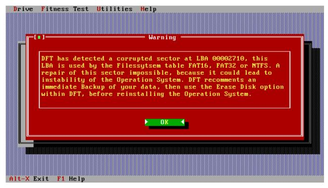
If for any reason, other than those stated above, DFT cannot complete the sector repair operation then the following test failure screen will be shown.
