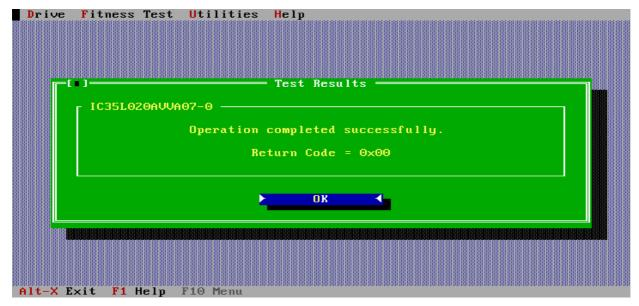
The next screen shows the conclusion of a test. In this case, the drive passed the DFT testing.
