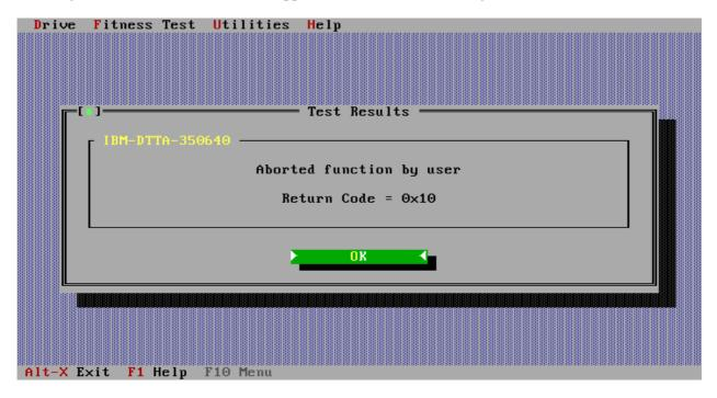
This says that testing has  $\underline{not}$  been completed, and is not a statement of either pass or fail. Testing must be restarted and run to completion in order to assess if there is a problem with the drive. The return code 0x10 is not an error.
