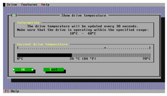
As a guide to evaluating if under normal operating conditions your system/enclosure will provide adequate cooling the **Test** option can be used. This test displays the current disk drive temperature (updated every 30 sec) during a random seek test, see the screen below. With this function you can simulate a high disk operation and determine the maximum temperature your drives will reach in your system and environment.
