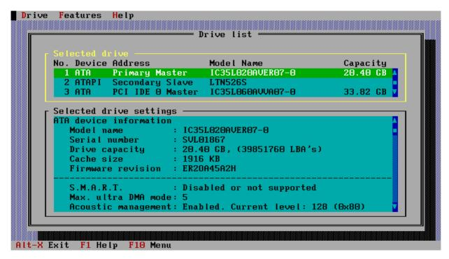
To navigate this screen the mouse can be used or alternatively use the cursor keys and the tab key. To modify a drive feature first select the drive using the mouse or cursor keys then select the pull down "Features" menu. This can be achieved with the mouse or <**Alt-F**> key combination. You will see a screen as shown below with the following options,
