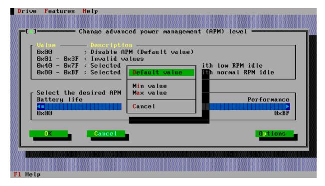
If the selected disk drive does not have or support changing the advance power mode then when this option is selected the following screen will be displayed.
