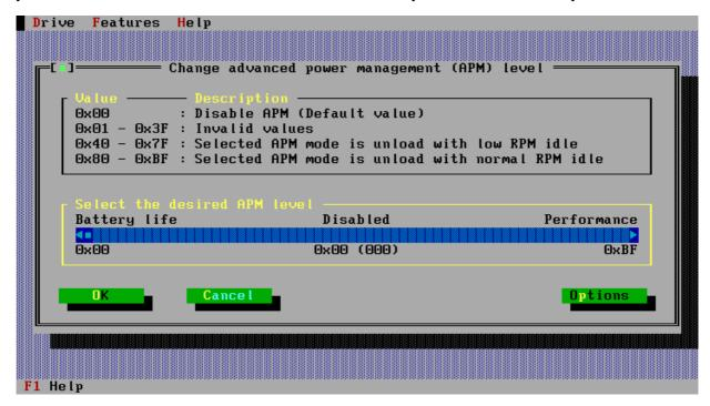
Selection of a pre-defined APM mode can also be made using the **options** button, as can be seen in the screen below.
