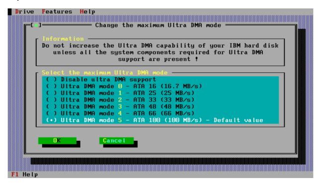
The current UDMA Mode setting of the selected drive will be highlighted, to change to a new setting use the cursor up/down keys to select the desired value, then tab to the **OK** button and press enter. When the change has been effected you will see the following screen, please follow the indicated instruction to complete the mode change.
