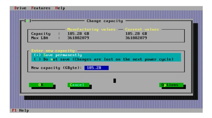
Some of the older Motherboards BIOS's don't support the larger capacity ATA drives, which are now available. The **Options** button provides a quick means of changing the drive capacity to just below the known boundary limits of 8GB and 32GB, it also provides a quick means of resetting the drive to its maximum capacity.
