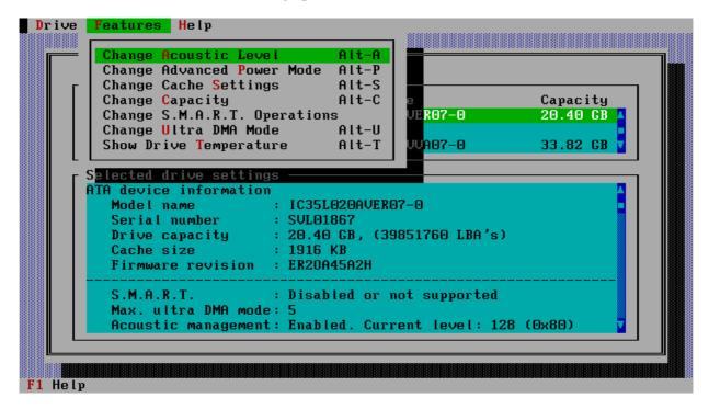
From the pull-down menu select the drive feature to be modified, for more detail on how to change each feature select from the links below.
