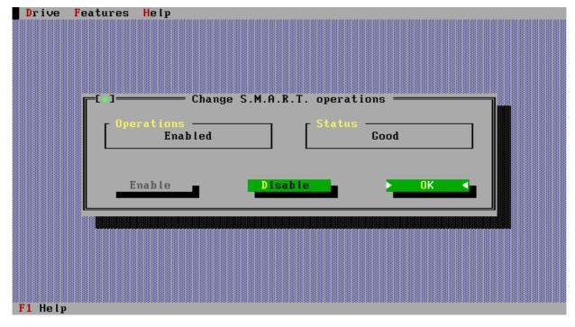
**Note:** on some system if SMART monitoring is enabled in the system BIOS then disabling SMART with this utility will be effective only until the next re-boot.
