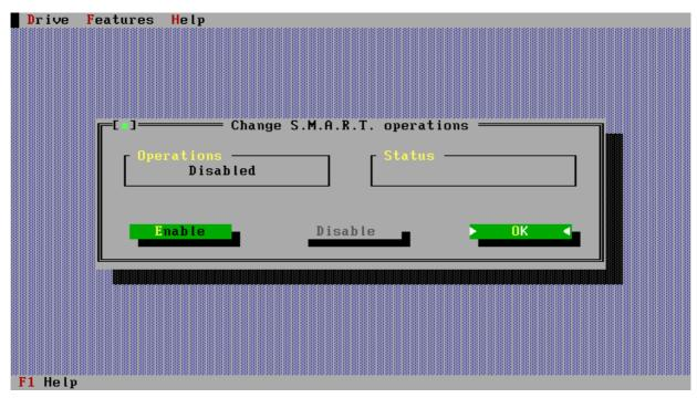
To enable/disable S.M.A.R.T., select the drive that you wish to change. Then from the Features menu select Change S.M.A.R.T. Operations, you will be presented with a screen similar to that shown above. S.M.A.R.T. can now be enabled or disabled on the selected drive by selecting the required function and hitting the enter key. When SMART is enabled you will see the status in the Status box.
