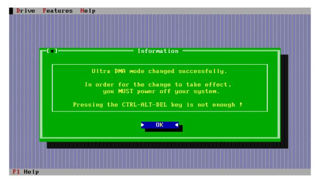
**NOTE**: This utility supports changing the UDMA setting of IBM drives only and only those drives on which the UDMA is a changeable parameter. The following IBM Hard disk drives support changeable UDMA modes, IBM DPTA (Deskstar 34GXP & 37GP) and IBM DJSA (Travelstar 20GN, 30GT & 32GH) and newer IBM ATA Hard Disk Drives.
